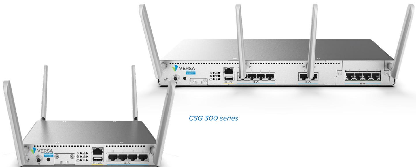
For rack-mounted deployments, the port side of the CSG300 series appliances is designed to simplify operations and accessibility and to improve visibility of device operational status and health. Status LEDs provide succinct visualization of the operational status of the device and of the Bluetooth, WLAN, and LTE connections.
